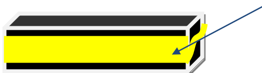
Diagram5. Sanding block with thick elastic band to hold both grades of abrasive in place.
